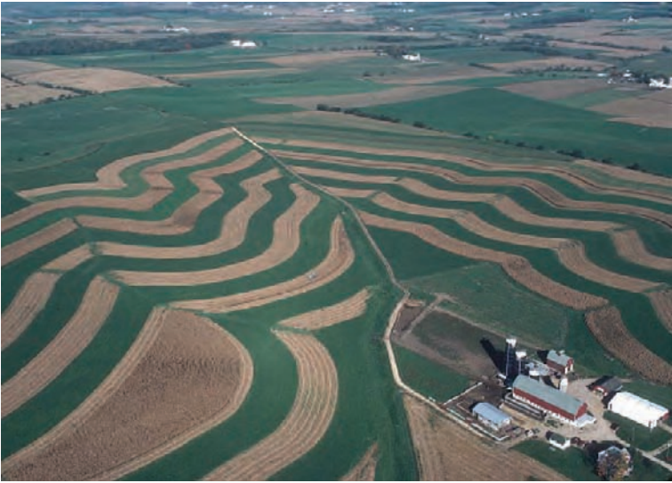
Plate 23 Contour stripcropping protects the soil from erosion and improves land aesthetics (Courtesy USDA-NRCS)
