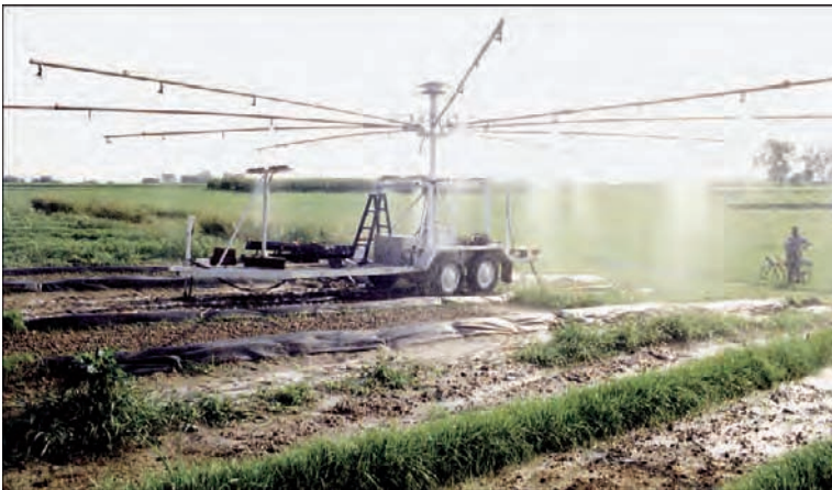
Fig. 2.6 The Swanson type rotating boom rainfall simulator (Photo by H. Blanco). The simulator booms are equipped with nozzles positioned at radii of 1.5, 3.0, 4.5, 6.0, and 7.6 m. Booms and nozzles rotate in a circle, and the wetted diameter is about 16 m
