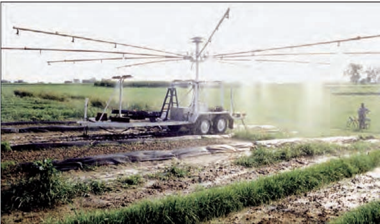
Plate 9 The Swanson type rotating boom rainfall simulator (Photo by H. Blanco). The simulator booms are equipped with nozzles positioned at radii of 1.5, 3.0, 4.5, 6.0, and 7.6 m. Booms and nozzles rotate in a circle, and the wetted diameter is about 16 m
